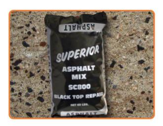
PARAGON BLACKTOP & ASPHALT PATCH is a blended mixture of slow cure liquid asphalt (SC800) meeting the ASTM D-2026 specifications; and aggregate composition and grading meeting Standard Specifications for Public Works Construction 1988 for Class D2 Asphalt Concrete.
