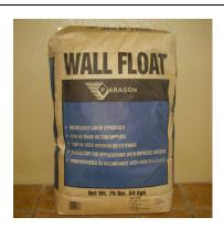
WALL FLOAT: is a pre-blened plaster mix specifically designed for the tile contractor. The control of mix ratio and quality of sand make it a superior product to job-site mixes. Wall Float is a blend of Portland Cement Type I-II-V (ASTM C 150), Lime Type-S (ASTM C 207), and washed and graded plaster sand (ASTM C 144) Specifications.
